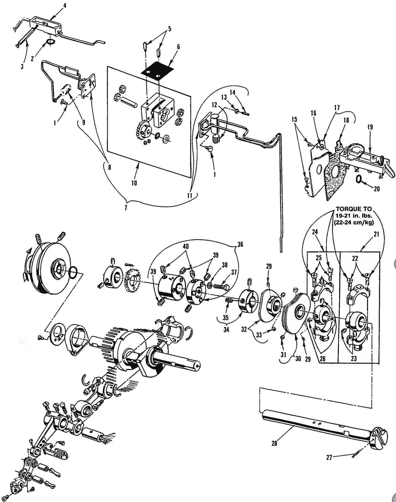
**MAIN SHAFT PARTS & MISCELLANEOUS OILING**
